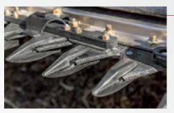
■ Knife heads, spline blocks, knife arms and hardware have been substantially beefed up to improve reliability and durability.
