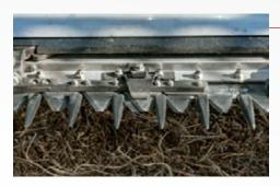
More robust knife heads include a factory-assembled and lubed knife arm and head vertically mounted, allowing adjustments as required to obtain the proper gearbox-to-cutterbar spacing.
