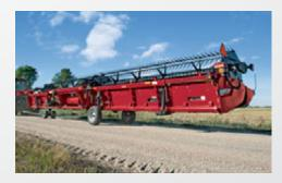
■ An industry-exclusive low-speed transport system (25 mph or less) allows the operator to deploy the transport package with the touch of a button, saving time when moving from field to field.
