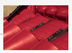
Grain-saving, patented CornLouvers™ direct grain back toward the auger to ensure loose grain makes it into the combine.
